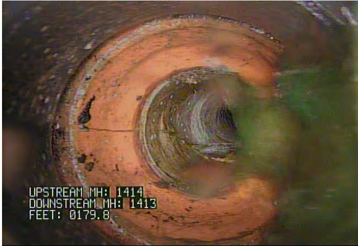
TFA - Tap, Factory Made: Active @ 179.8 ft. DYE PRESENT
